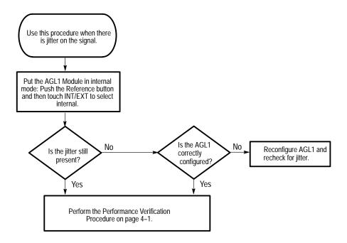
Figure 6–7: Flowchart for jitter on signal
