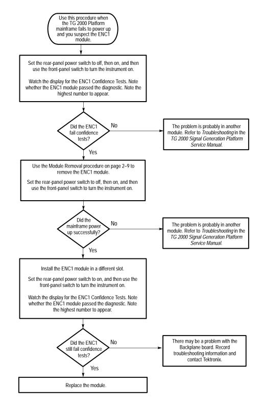
Figure 6–5: Flowchart for failure to power up
