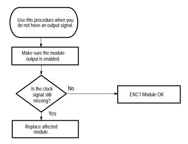
Figure 6-6: Flowchart for missing output signal
