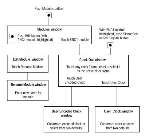
Figure 2–7: Basic menu structure for the ENC1 module
