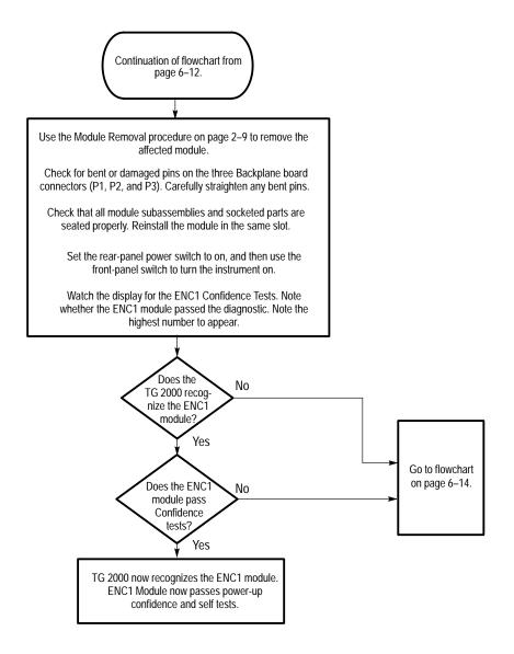
Figure 6-3: Flowchart for checking the current module installation slot
