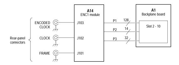
Figure 9–1: ENC1 module connections
