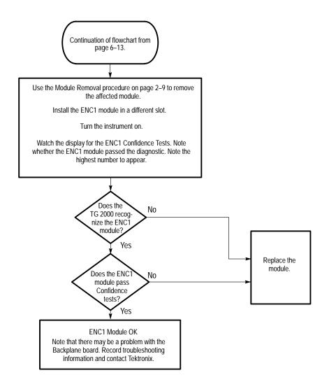
Figure 6-4: Flowchart for checking the module in a different slot
