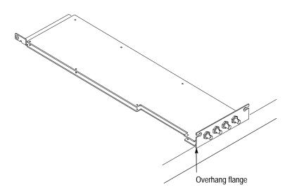
Figure 6–1: Position the shield flat on the work surface
