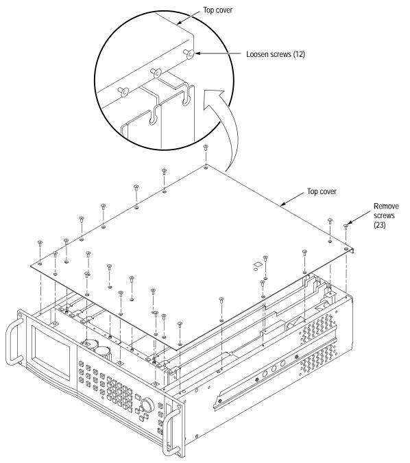
Figure 2–2: Top cover removal
